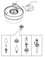
Reinstall the bottom plate and tighten the 3 screws.
