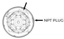
Attach the spring cable and tighten the 6 screws to secure the cover.
