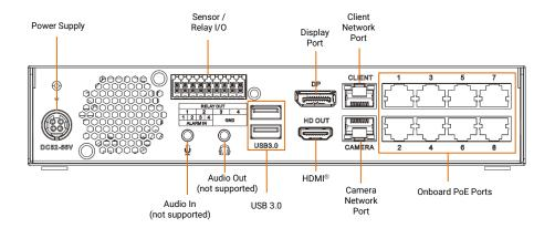
WARNING The Camera Network Port is equipped with a DHCP server and intended for use only with a dedicated independent camera network on its own network switch. Connecting the Camera Port to a network with another DHCP server will cause significant network issues.
